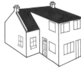
An inappropriate extension which dominates the existing house.
