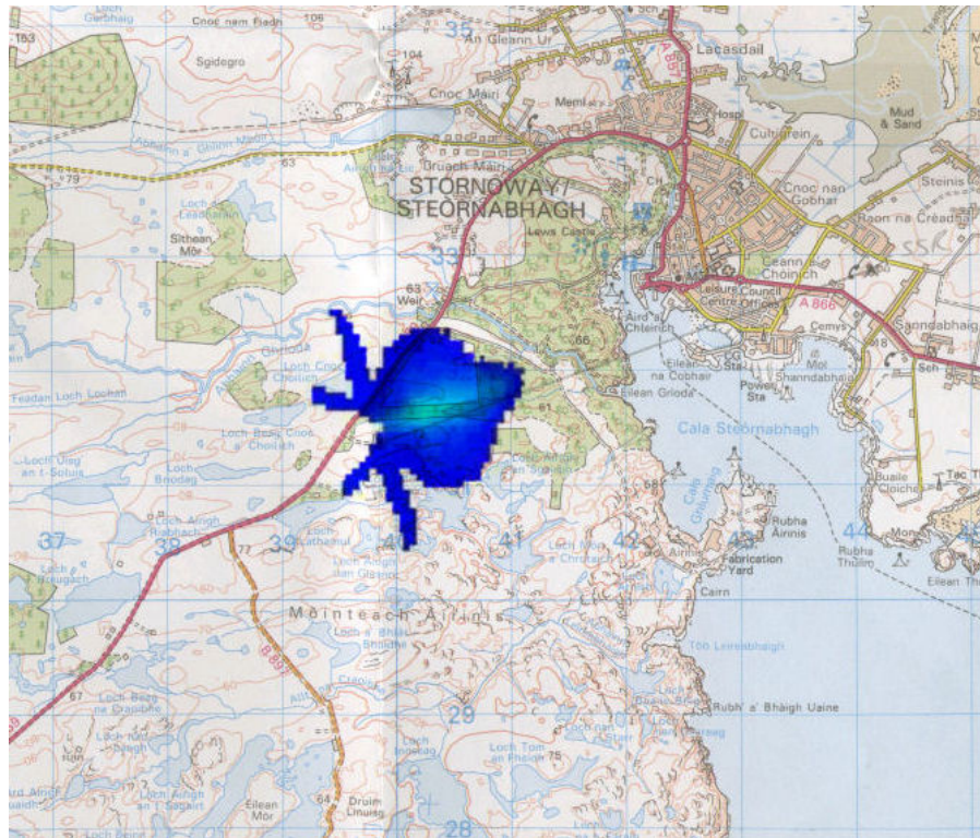
Figure 3-3; Impact zone for a Vestas V29 turbine on a 30 m tower using the 90% turbine scattering level.
