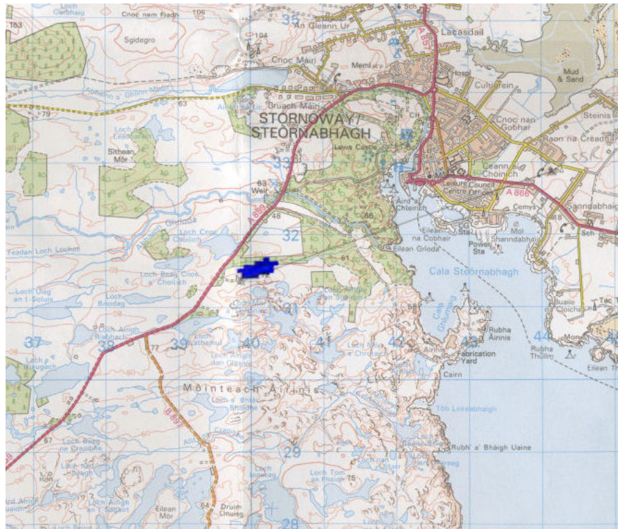
Figure 3-4; Impact zone for a Vestas V17 turbine on a 23 m tower using the 90% turbine scattering level.
