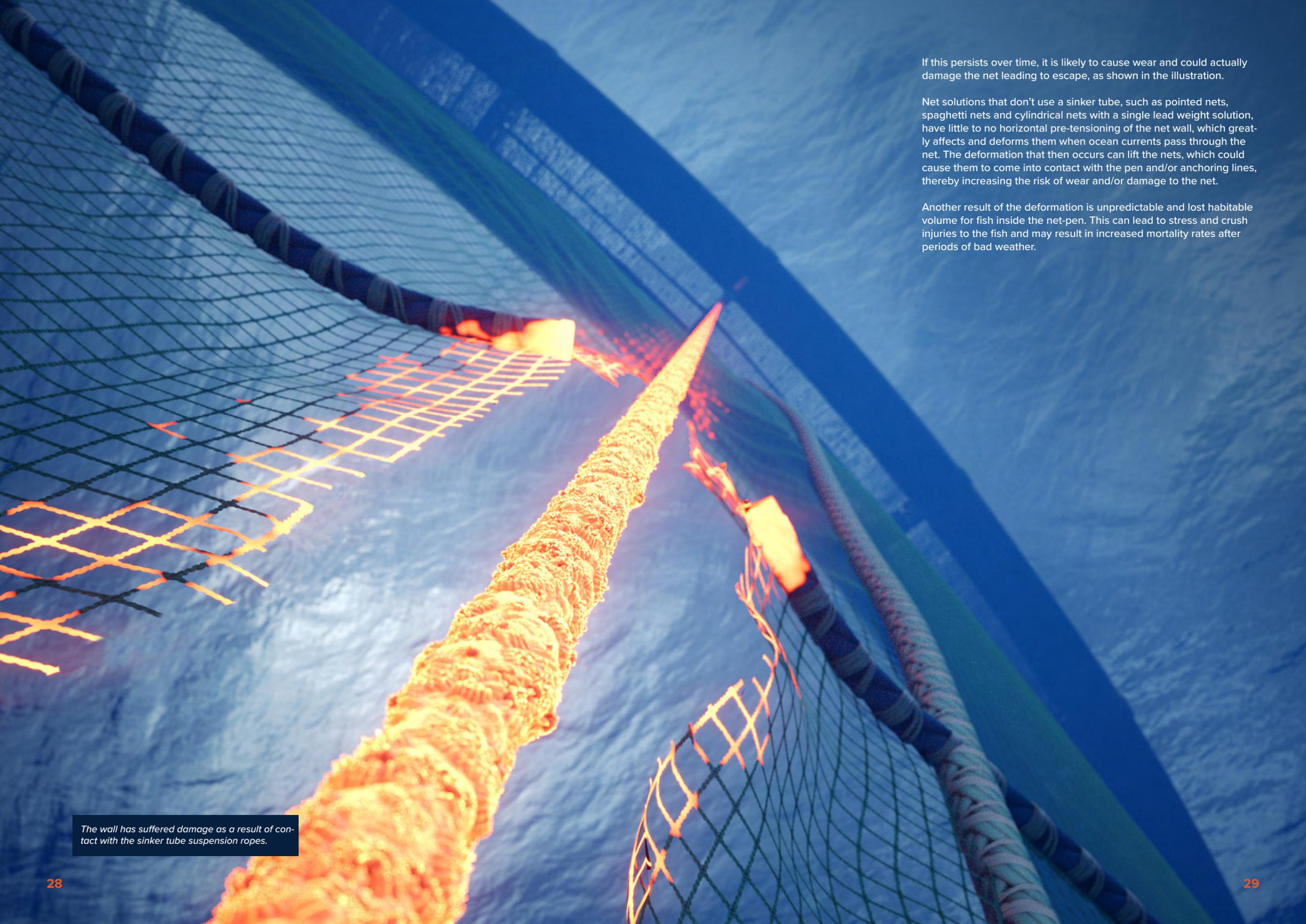
If this persists over time, it is likely to cause wear and could actually damage the net leading to escape, as shown in the illustration.
