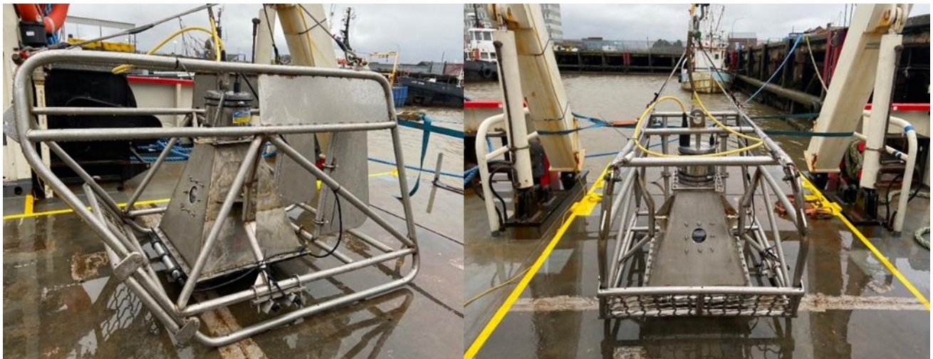
Plate 2 OEL's bespoke drop-down camera and deployment frame.
